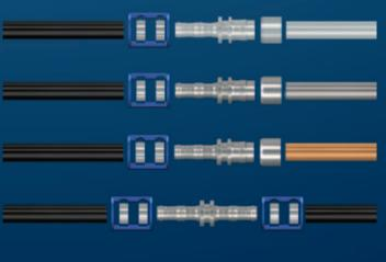
What can you connect using LOKRINGs? There's a simple answer to that: All the metal tubes used in air-conditioning and cooling technology with a wall thickness of 0.5 mm to 1.5 mm. There is almost no limit to the combination variations here. One rule of thumb is: If at least one of the tubes to be connected is made of aluminium, an aluminium LOKRING must be used as well. In all other cases, a brass LOKRING is used.
