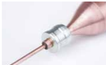
07. Dryer to Capillary Tube
